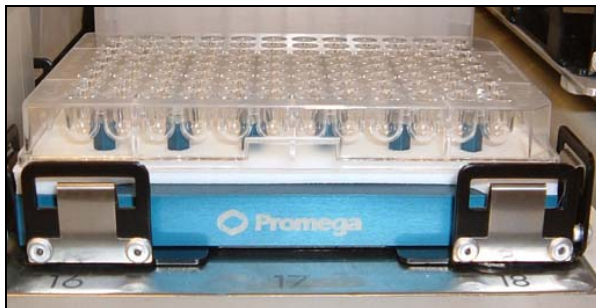
Figure 8. MagnaBot Assembly. Shown is the 24-post magnet with spacer and Greiner U-bottom plate at deck position G16.
